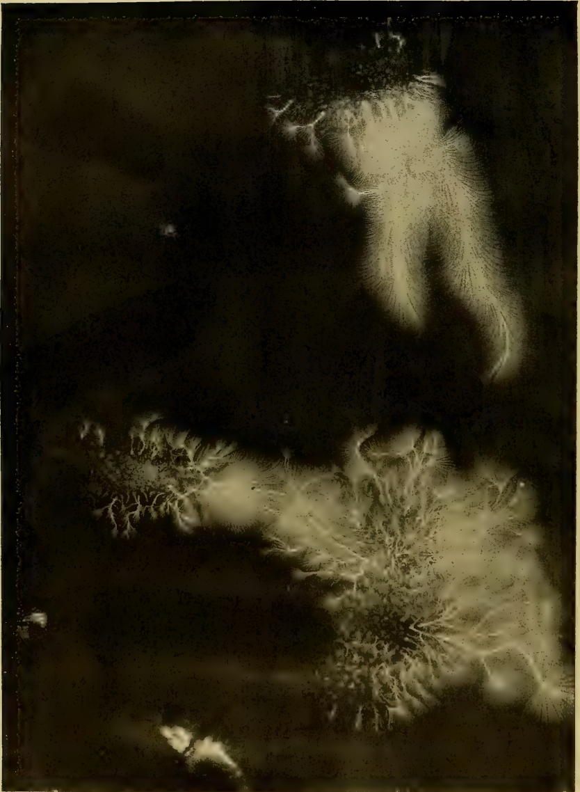
PLATE 2.—Photograph of Spark Discharge on Film. This plate illustrates the effect of an electric discharge of accidental occurrence just prior to connecting a tube in circuit. The photographic plate was on the base of the tube-holder: the patient's hands were on the plate, and the wires from a ten-inch coil were supported by a high stand with their free ends resting on the table within an inch or two of the plate. The current was accidentally turned on for a few seconds while preparing for the exposure. The negative wire was at the lady's right hand. She felt a shock, but there was neither spark nor disruptive discharge seen. No trace of the current could be detected afterward on the plate-envelope. The print shows that the spark reaching the film was a small discharge. Beautiful studies of these tree-fern-like tracings on sensitive films may be made at will by any operator, and it does not require much of a current to fill the face of an 8 x 10 plate with wonderful markings. Each pole makes its own peculiar tracing, and when both discharges meet the front and back of the plate at the same time a merging of effects results which can easily be identified by one familiar with these pictures. (Rebman, Ltd.)
